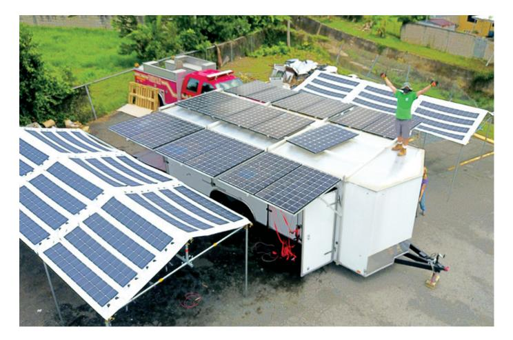
Mobile solar+storage trailer designed by Footprint Project with funding from Empowered by Light and assembled in Puerto Rico by Sail Relief Team and Humacao Fire Station. Courtesy of Footprint Project
