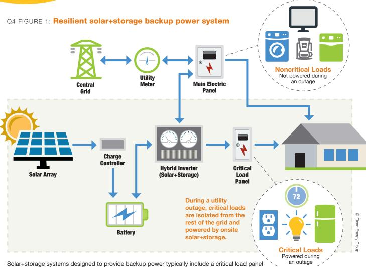
and a transfer switch to disconnect from the utility grid. The transfer switch is often incorporated as a component of the system's hybrid inverter, shown here in a DC-coupled configuration. When an outage occurs, the transfer switch isolates the solar+storage system from the grid along with the critical load panel. Any devices served by the critical load panel will continue to be powered by solar+storage, while those served by the main electric panel will not be powered during an outage.
