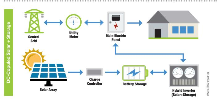
Solar and energy storage systems can be integrated together through either AC- or DC-coupled configurations. The main difference between AC and DC coupling is that, in a DC-coupled system, solar and storage components share a hybrid inverter, whereas, in AC-coupling, solar and storage components each have their own separate inverters.
