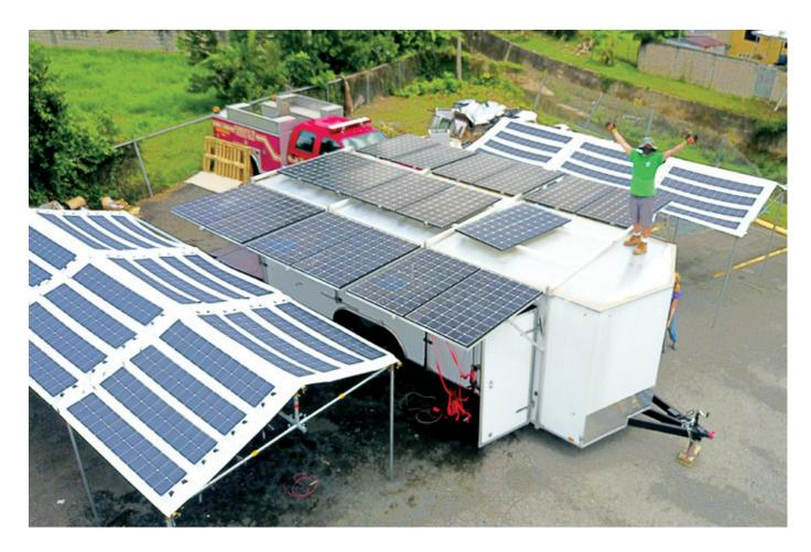
Mobile solar+storage trailer designed by **Footprint Project** with funding from Empowered by Light and assembled in Puerto Rico by Sail Relief Team and Humacao Fire Station.
