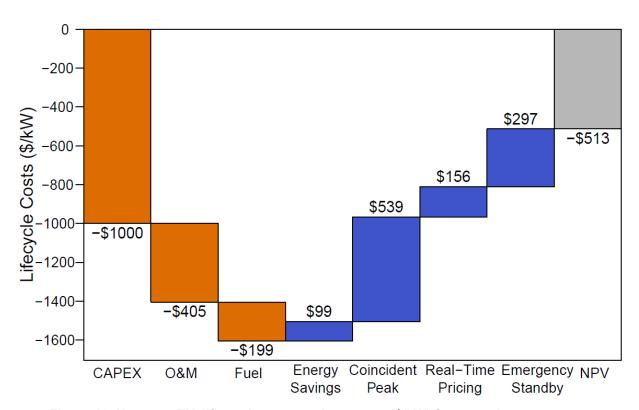
Figure 10. Houston, TX, life-cycle costs and revenues (\$/kW) for natural gas generator.
