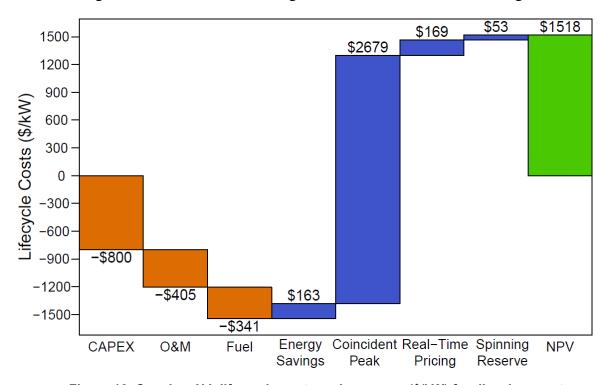
Figure 13. Camden, NJ, life-cycle costs and revenues (\$/kW) for diesel generator.
