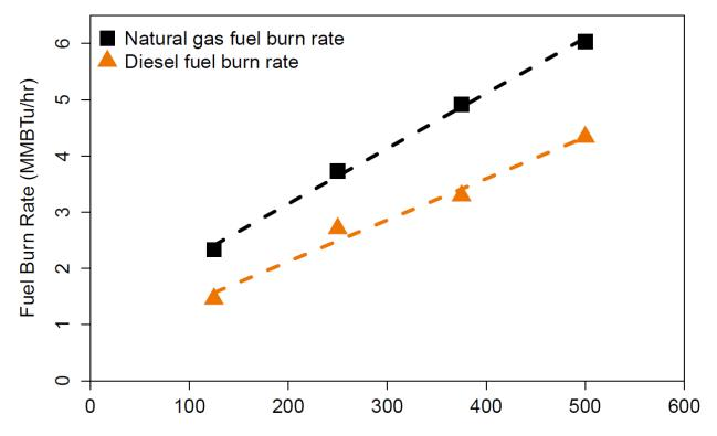
Figure 7. Fuel consumption for modeled generators.
