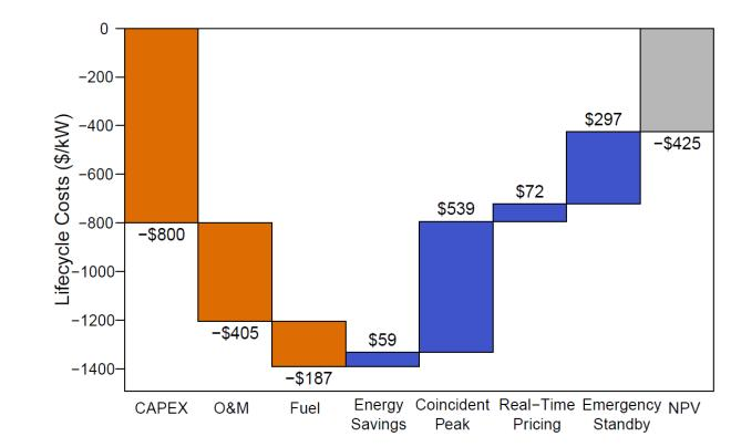
Figure 9. Houston, TX, life-cycle costs and revenues (\$/kW) for diesel generator.
