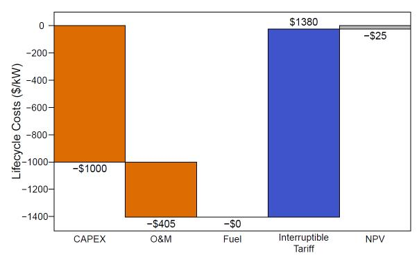
Figure 12. Orlando, FL, lifecycle costs and revenues (\$/kW) for natural gas generator.
