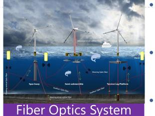
Fiber Optics System for a Real-Time Monitoring
