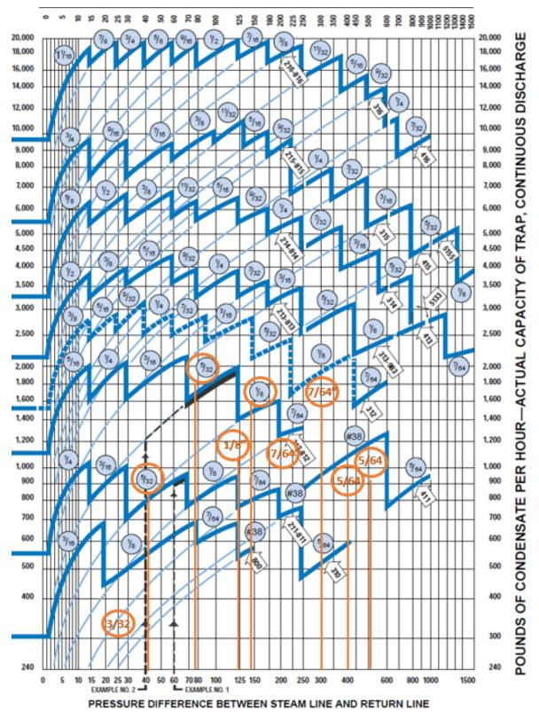
Figure 5: Plot of gauge pressure and orifice size.
