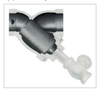
Figure 3: Strainer with blow-off valve to the bottom.
