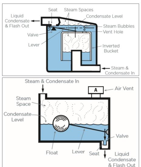
Figure 2: Two common types of steam trap: Inverted bucket steam trap (top) and float and thermostatic steam trap (bottom).
