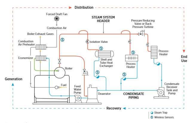
Figure 1: Steam system schematic.
