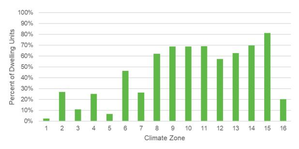
Figure 15: Percent of new construction multifamily projects up to three habitable stories with refrigerant charge verification.
