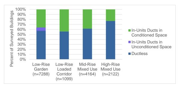
Figure 10: Distribution of duct type and location for sample of California multifamily projects.
