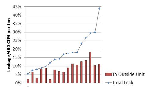
Figure 14: Duct leakage for a sample of multifamily projects one to three habitable stories built under the 2005 Title 24, Part 6 code.
