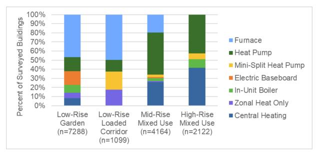
Figure 8: Distribution of HVAC heating system type for sample of California multifamily projects.
