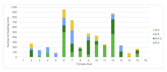
Figure 13: Distribution of duct insulation R-value by climate zone for ducts in conditioned space in multifamily projects up to three habitable stories.
