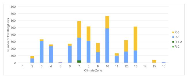
Figure 12: Distribution of duct insulation R-value by climate zone for ducts in unconditioned space in multifamily projects up to three habitable stories.
