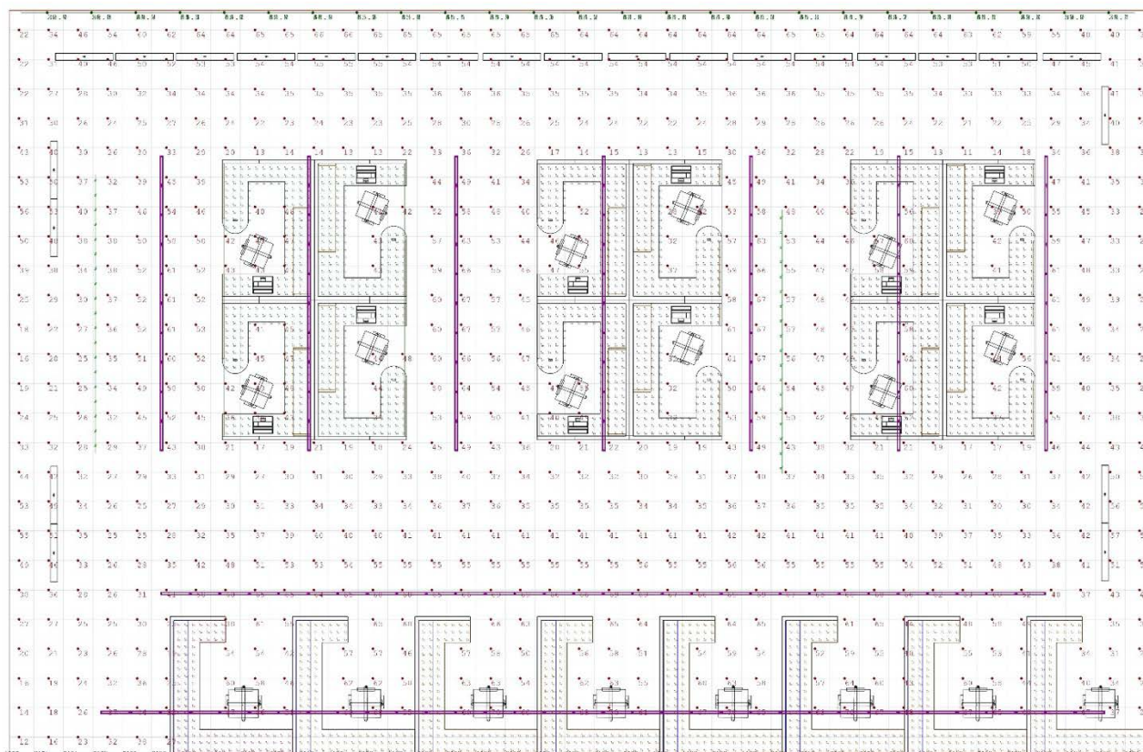
Figure 48: Plan View 2022 Design A2 (Direct Indirect Pendant Lighting Providing Task and General Lighting).
