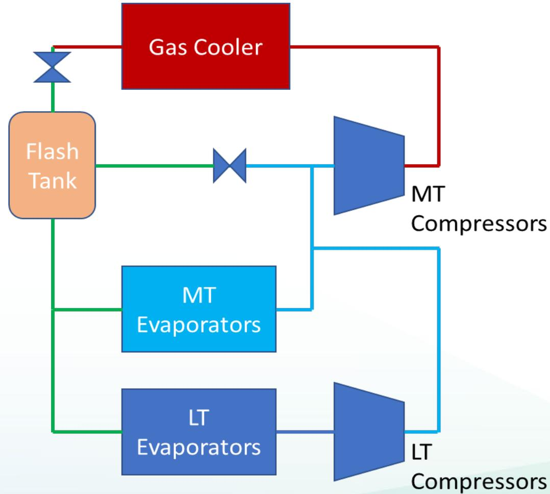
Transcritical CO<sub>2</sub> Booster Refrigeration System Diagram
