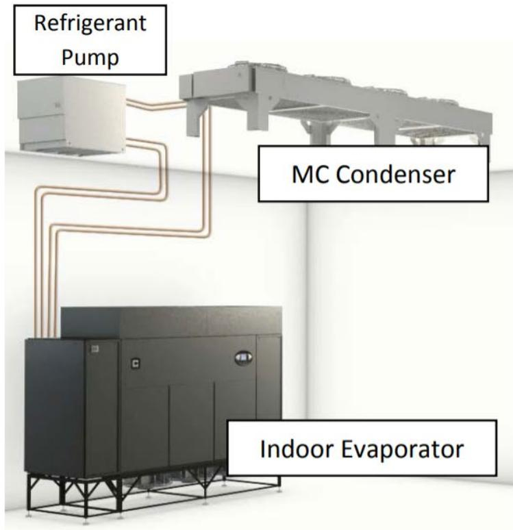
Fig 1 - System Component Layout
