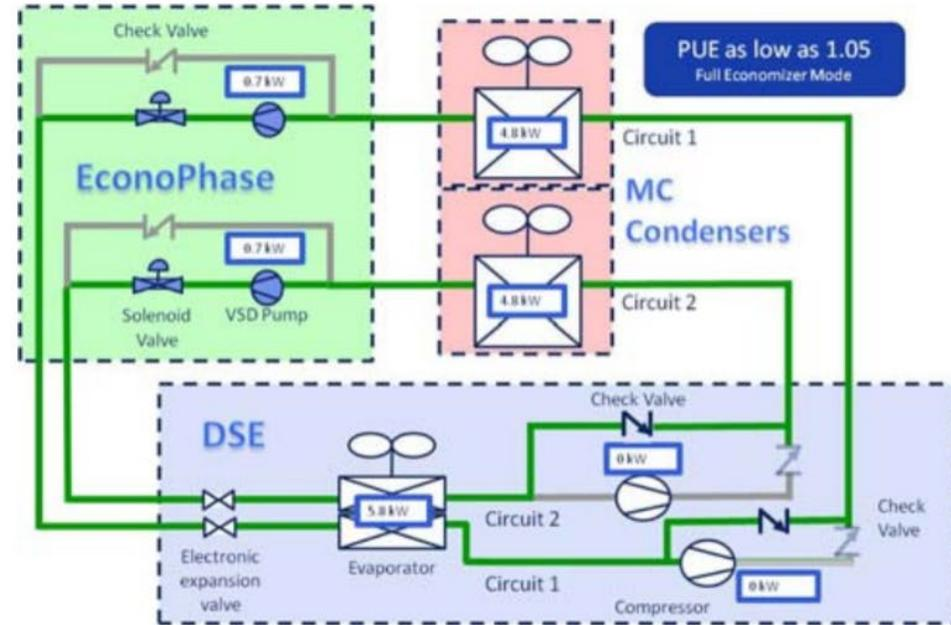
Fig 2 - System Flow Diagram
