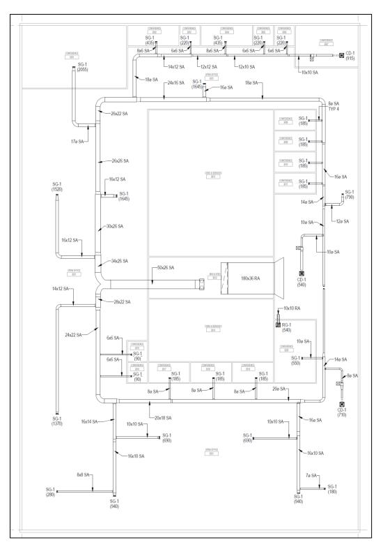
Figure 12: Large Office VAV Proposed Design.
