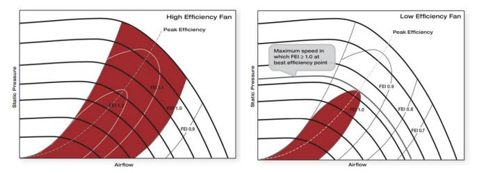
Figure 4: High and low efficiency fans with FEI ratings.
