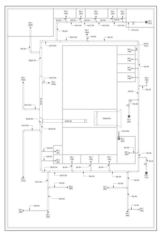
Figure 13: Large Office VAV Standard Design.
