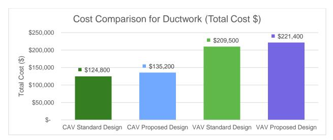
Figure 8: Large Office ductwork total cost (\$) for a CAV and a VAV system.
