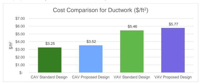
Figure 9: Large Office ductwork cost (\$/ft2 building floor area) for a CAV and a VAV system.
