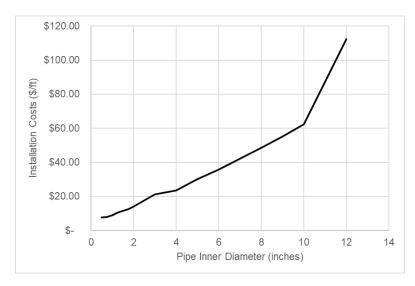
Figure 11: Piping installation costs.
