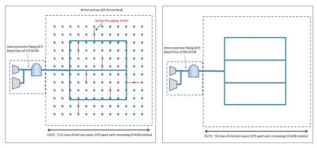
a) Prototype 1, Rated flow 579 cfm
