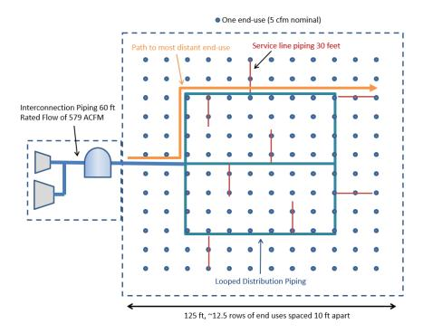
Figure 7: Piping layout of Prototype 1 showing path of greatest frictional pressure loss.
