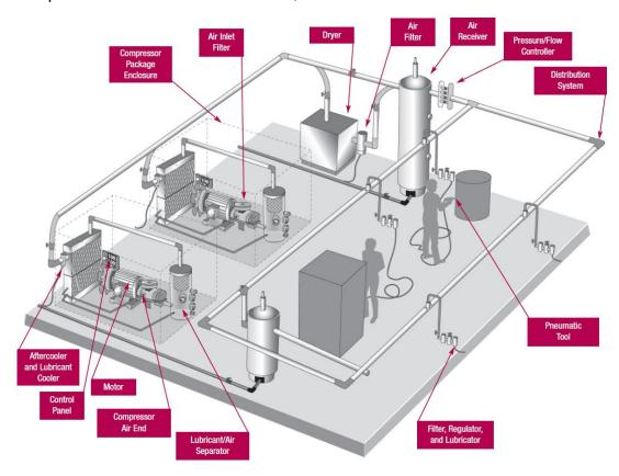
Figure 2: Simplified compressed air system.
