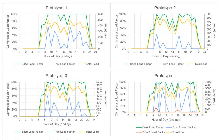
Figure 5: Prototype weekend load profiles.
