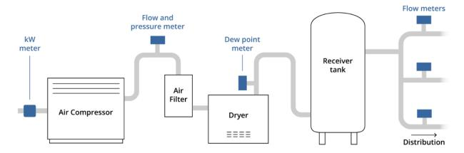
Figure 1: Example monitoring points
