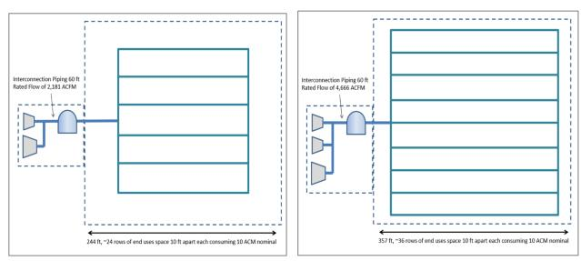
c) Prototype 3. Rated flow 2,181 cfm
