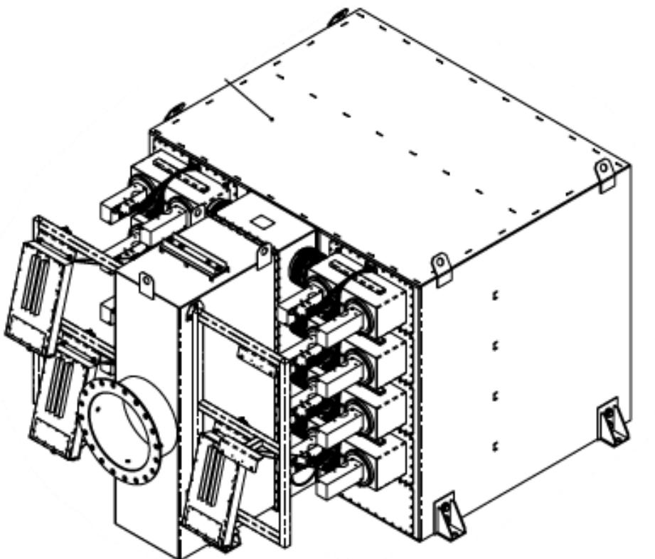
**Active Diesel Particulate Filter****Intelligent microprocessor control****PM reduction up to 93%****Low back pressure**
