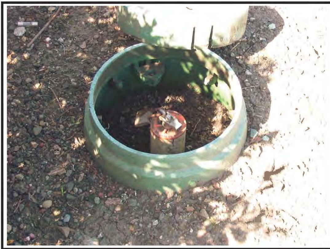
Photograph 15: Standing near the southwest corner of the site and looking at the wellhead for monitoring well M-4. Wellhead is located inside an irrigation system valve box, not a groundwater monitoring well box.
