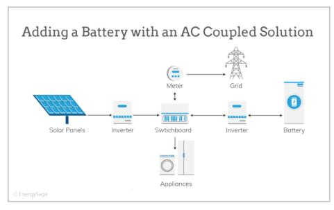
Figure 2: Battery storage system paired with solar PV.
