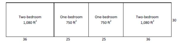
Figure 37: Low-rise garden first and second floor plan.
