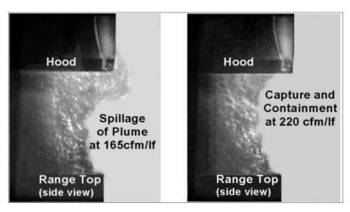
Figure 7: Illustration of range hood plume spillage at different airflow rates. Source: (ASHRAE 2011).
