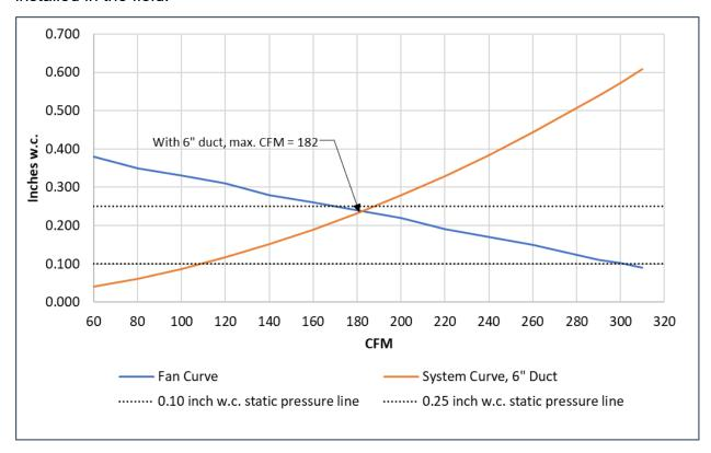
Figure 10: Typical kitchen range hood system and fan curves.
