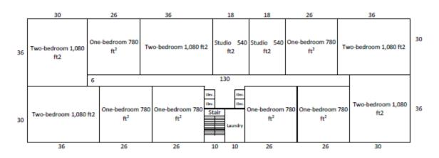
Figure 43: High-rise mixed use second through tenth floor plan.
