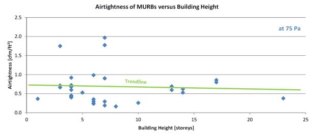
Figure 35: Airtightness of multifamily buildings versus building height Source: (RDH, Air Leakage Control in Multi-Unit Residential Buildings 2017)
