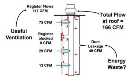
Figure 12: Ventilation duct leakage, with hypothetical flow rates.
