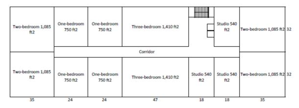
Figure 39: Low-rise loaded corridor second and third floor plan.
