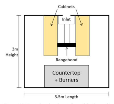
Figure 45: Test chamber front view with dimensions
