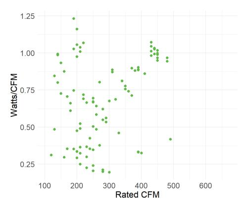
Figure 22: Kitchen range hood power per unit of flow.
