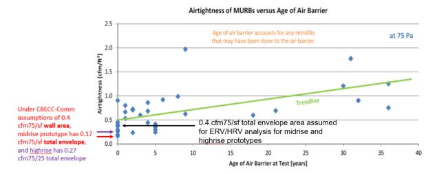
Figure 34: Airtightness of multifamily buildings versus age of air barrier Source: (RDH, Air Leakage Control in Multi-Unit Residential Buildings 2017)
