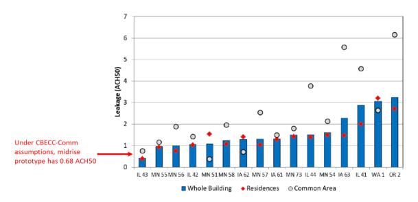
Figure 32: Multifamily leakage (measured at the whole building level) compared to CBECC-Comm infiltration assumption
