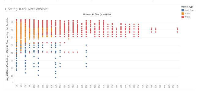
Figure 14. Net Sensible Recovery Effectiveness of E/HRVs in AHRI database (Courtesy Red Car Analytics)
