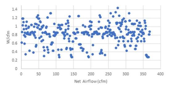
Figure 15. Fan Efficacy of HRVs and ERVs in HVI Database
