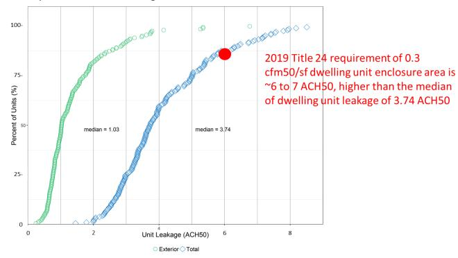
Figure 33: Leakage results in multifamily dwelling units: Total envelope leakage and exterior leakage only
