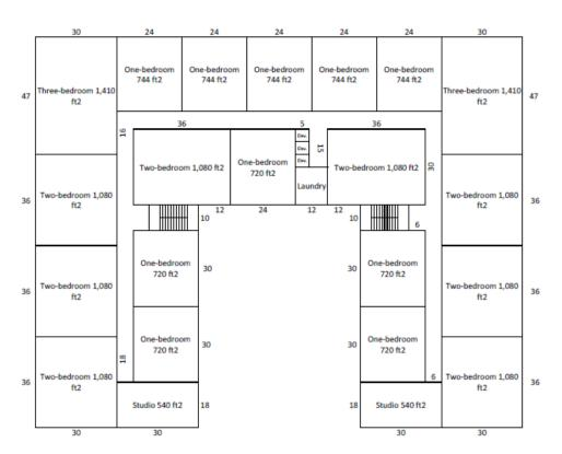
Figure 41: Mid-rise mixed use second through fifth floor plan.
