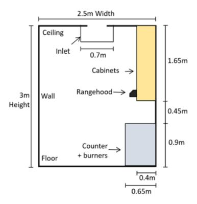
Figure 44: Test chamber side view with dimensions
