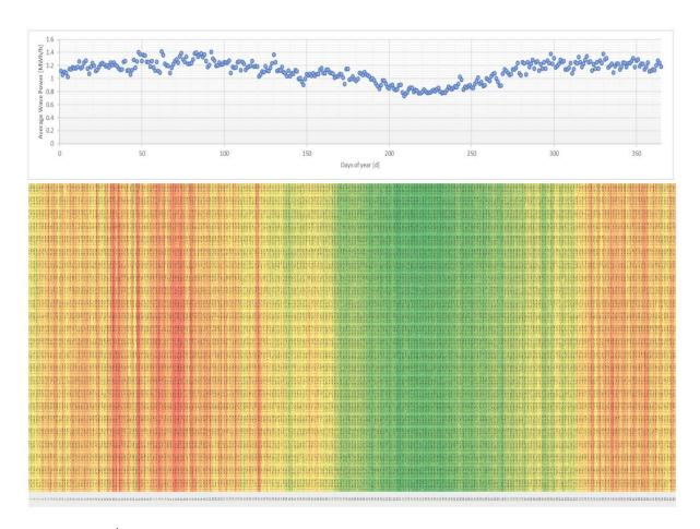
**Figure 1**<sup>‡</sup> Daily average and hourly output of CalWave wave energy convert at central California case study site for Southern California Edison, Vandenberg. Source: CalWave internal analysis based on NBDC wave data.
