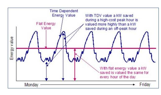
TDV values for electricity tend to favor designs that reduce cooling loads, when grid costs are highest. TDV values for natural gas tend to disfavor electrification because of the low cost of natural gas.
