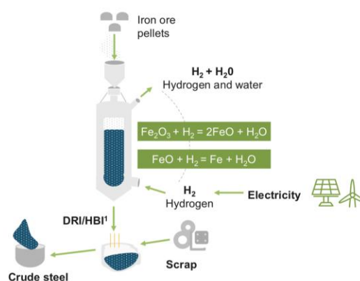
Figure 7-6 Hydrogen-Based Ironmaking Process
