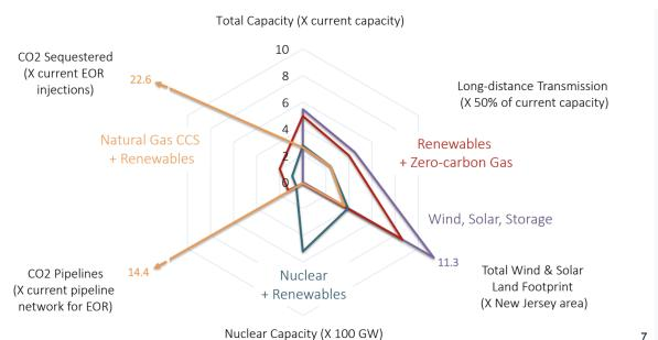
Figure 10: National buildout required for 100% carbon-free electricity, by technology. Source: J. Jenkins, *Critical bottlenecks in decarbonization of the U.S. electricity grid*, Jesse D. Jenkins, PhD, Princeton Rapid Switch Workshop (June 12, 2019), used by permission of author
