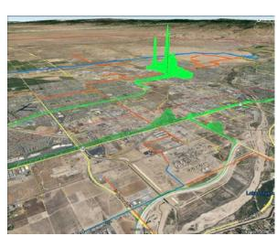
Methane above ambient (green), distribution (orange) and transmission (blue) pipelines
