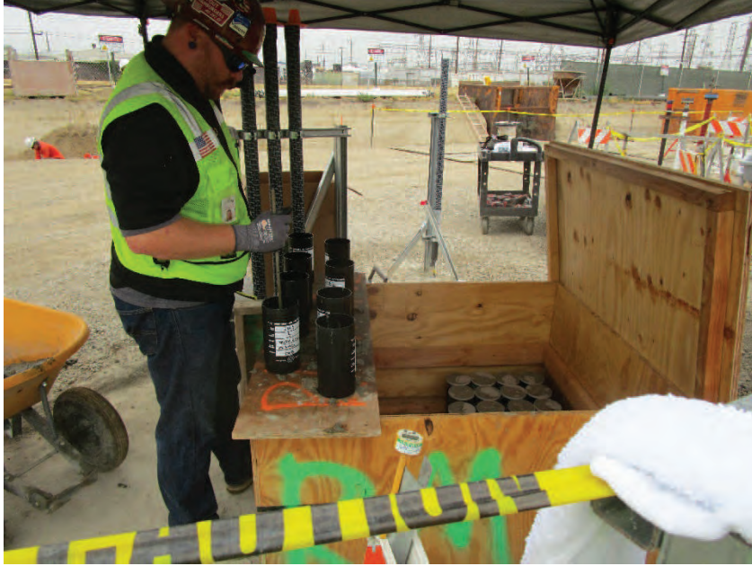
6/25/2019: CTG2 Concrete Strength Cylinder Casting
