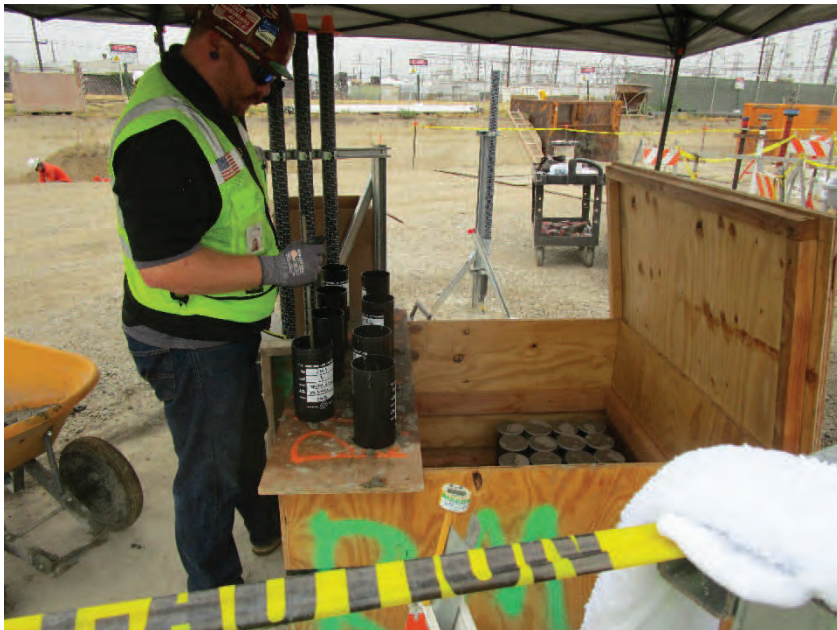
6/25/2019: CTG2 Concrete Strength Cylinder Casting
