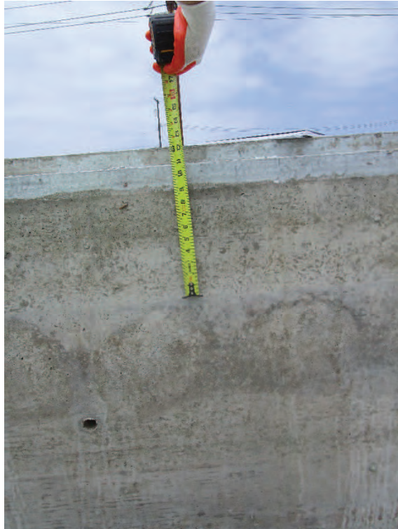
6/24/2019: GSU Pedestal Cold Joint Elevation Measurement 1
