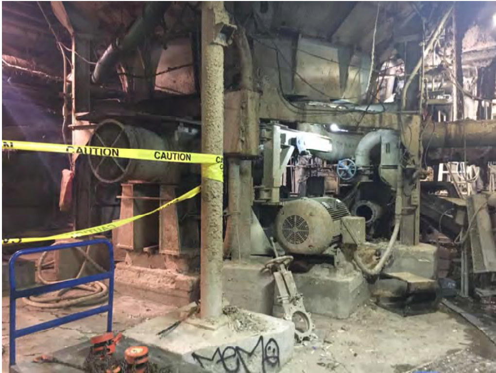
Photo 55: The site, facing southeast within the below-ground basement area. One of three interior pulper vessels (this is the filler pulper) with sub-grade containment (bottom-center) are located in this region of the basement. Oil reservoirs are located along the sides of each pulper.
