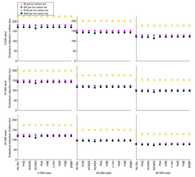
Fig. 4 Annual  $CO_2$  emissions (million ton) in Texas for the year 2012 in the base case with an 8.2-GW minimum-dispatchability requirement. Figure panels correspond to different wind- and solar-penetration levels, which are indicated at the left-hand side and bottom, respectively, of the figure. Source data are provided as a Source Data file
