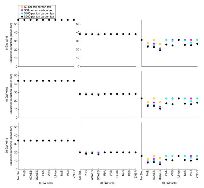
Fig. 3 Annual CO<sub>2</sub> emissions (million ton) in California for the year 2012 in the base case with a 7.0-GW minimum-dispatchability requirement. Figure panels correspond to different wind- and solar-penetration levels, which are indicated at the left-hand side and bottom, respectively, of the figure. Source data are provided as a Source Data file
