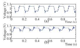
Fig. 8: Normalized voltage in a sub-transmission bus in Scenario-1: (a) Without smart inverters, and (b) With smart inverters.
