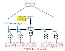
Fig. 6: Distribution system with distributed energy storage in Scenario-2.
