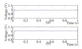
Fig. 9: Normalized voltage in a sub-transmission bus in Scenario-2: (a) Without smart inverters, and (b) With smart inverters.
