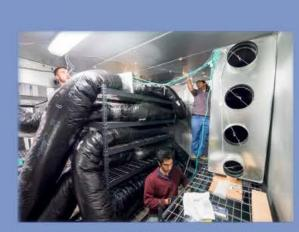
**Ductwork Setup in WCEC Testing Chamber**
