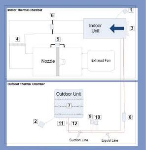
Schematic of Test Setup
