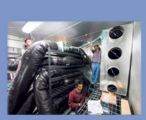
Ductwork Setup in WCEC Testing Chamber
