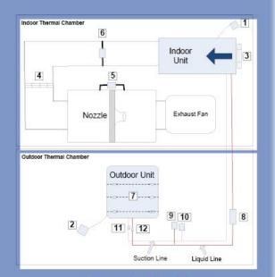
Schematic of Test Setup
