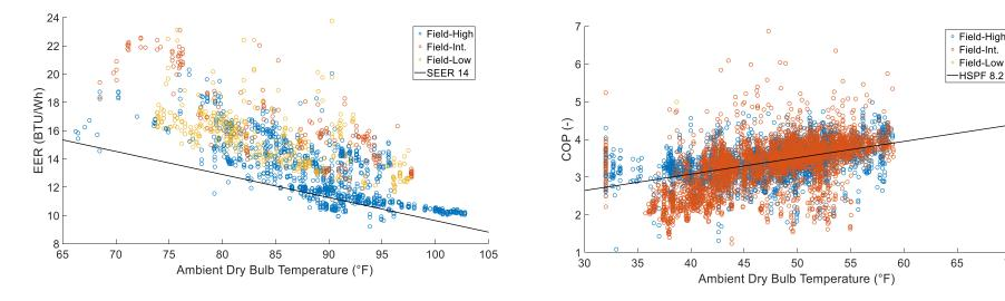
Unit cooling efficiency results @ PG&E site
