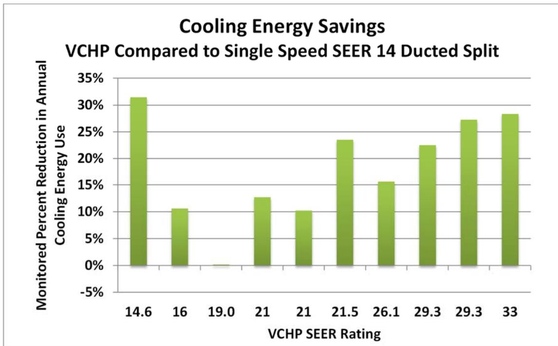
Figure 3: VCHP Cooling Energy Relative to SEER 14 Single Speed System, by SEER Rating
