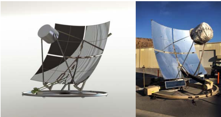
Figure 1: Deployable 250,000 BTU SHW system. The energy storage device is the grey cylinder located opposite the collector mirror.
