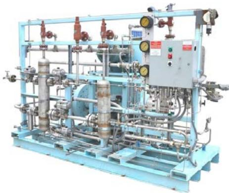
**Figure 12-A.** Used PDC Machines two-stage Hydrogen diaphragm compressor owned by AASI. It was previously installed in a wind-to-Hydrogen plant in Idaho. It will be refurbished for this project, to load the "tube trailer" from the low-pressure electrolysis stack output, at ~ 3,000 psi.
