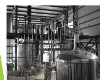
Syngas is cleaned, cooled, and sent to a bioreactor that converts it to a crude ethanol/water mixture;
