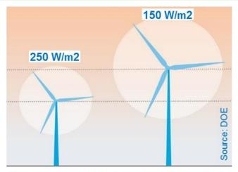
Current turbine size with contemporary rotor Future turbine with larger size advanced technology rotor
