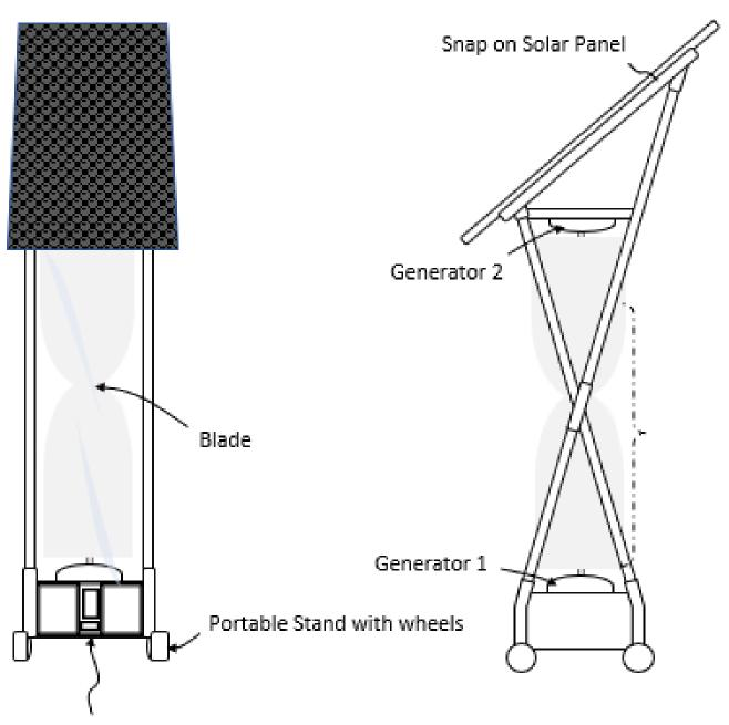
Battery Compartment including Charger, USB Ports, Smart Plugs, Wireless Controller with WIFI/Bluetooth, GPS (linked to weather forecast), and Smartphone Monitoring
