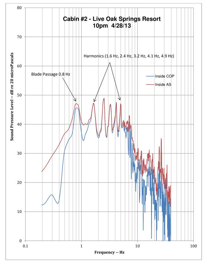
Figure C - 3 Live Oak Springs Resort - Cabin #2 - Comparison of Autospctrum and COP
