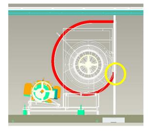
In this generic unitary air conditioner example, an increase in scroll width of 3.5" interferes with the fan wall.
