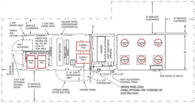
Top view of a 70 ton Intellipak 1 unitary air conditioner
