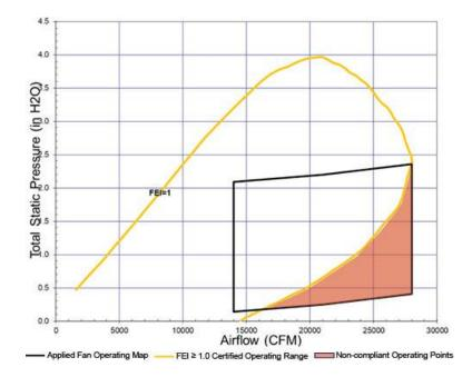
Just as with the supply fan, replacing the current 20" FC relief fans with 22" FC fans or 20" AF fans, as would be needed to improve the FEI, will require system re-optimization. Seeing as the relief fans are even more space-constrained than the supply fans in the 70 ton Intellipak 1, there is an increased
