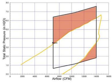
— Applied Fan Operating Map \_\_\_\_\_ FEI ≥ 1.0 Certified Operating Range \_\_\_\_\_ Non-compliant Operating Points
