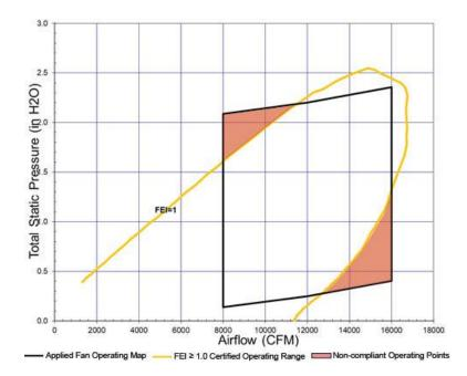
Similar to the relief fan in the 70 ton Intellipak, a new fan will need to be selected to accommodate the needed operating map, likely a 20" FC fan or 18" AF fan. Space constraints are similar for the relief
