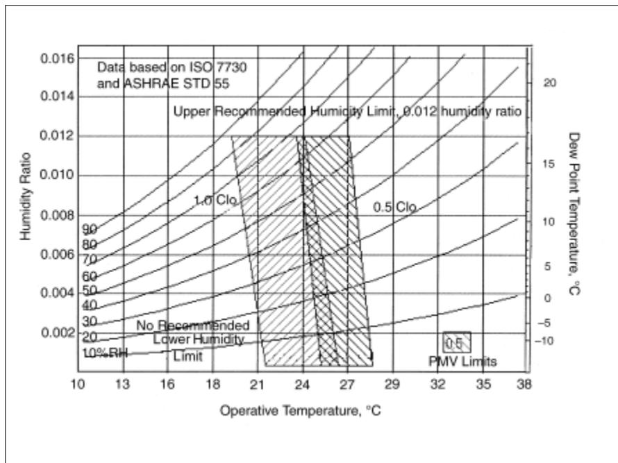
**Figure 7B.2.1 ANSI/SHRAE Standard 55-2004: Thermal Environmental Conditions for Human Occupancy**
