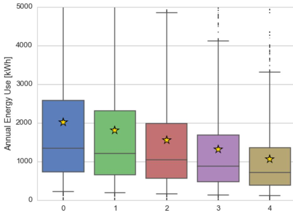
**Figure 7.3.3** Range of Annual Energy Use for Portable Air Conditioners in the Commercial Sector
