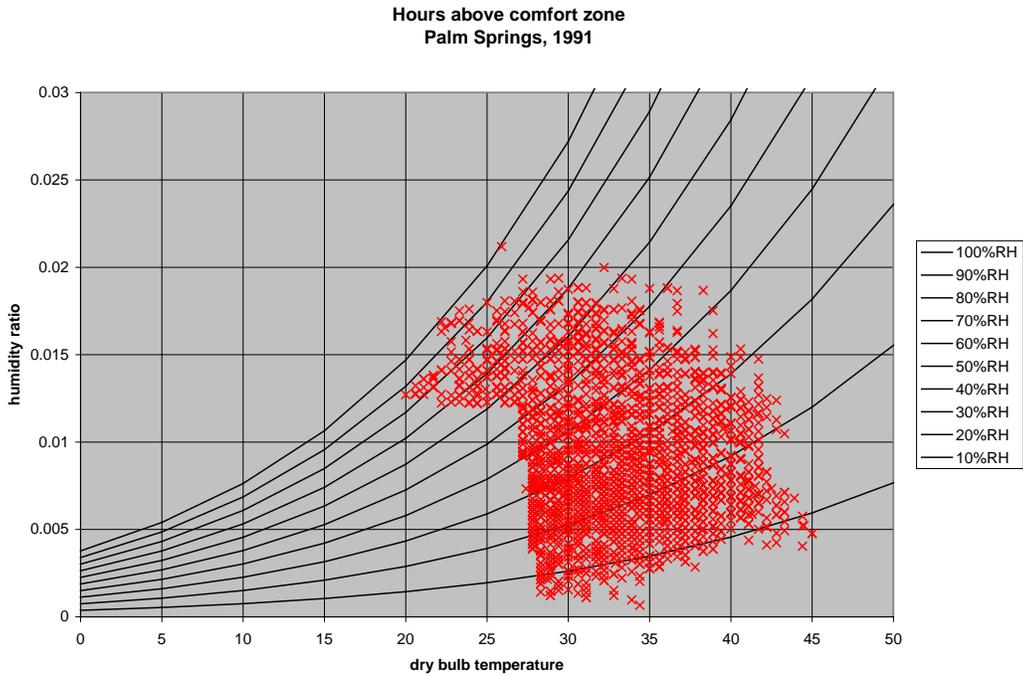
**Figure 7B.3.2 Hours that Exceeded ASHRAE Standard 55 Comfort Zone in Palm Springs CA, 1991**
