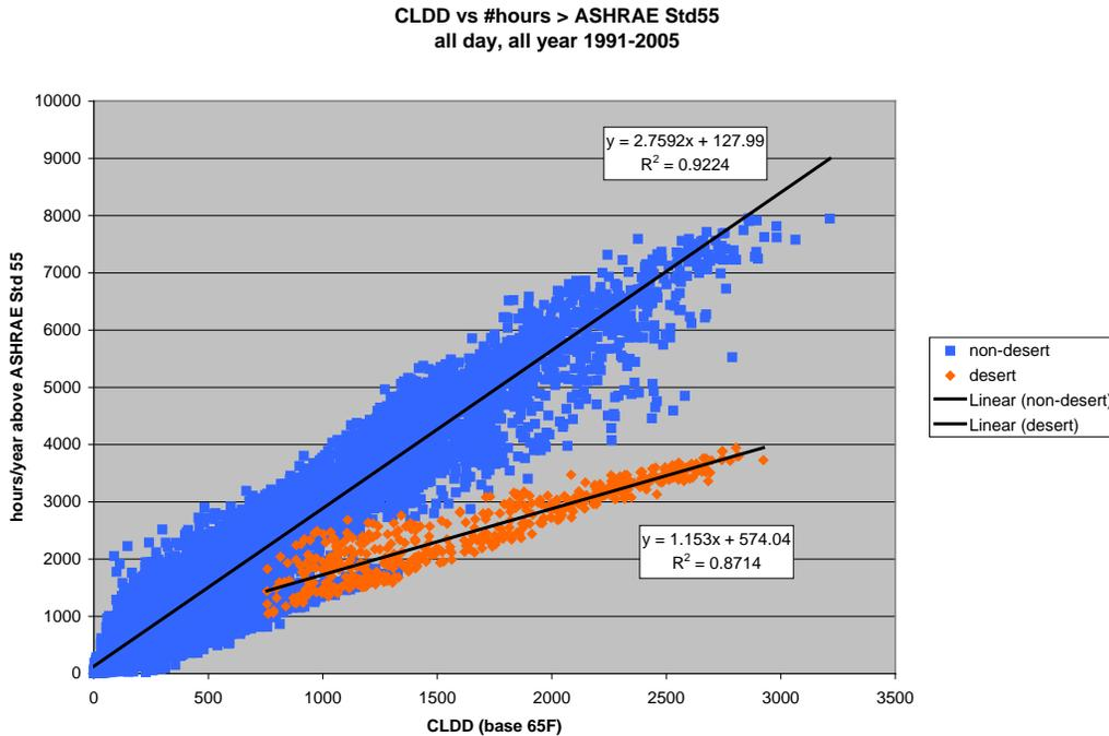
**Figure 7B.4.1 Hours that Exceeded ANSI/ASHRAE Standard 55 Comfort Zone as a Function of Cooling Degree-Days, Continental United States**
