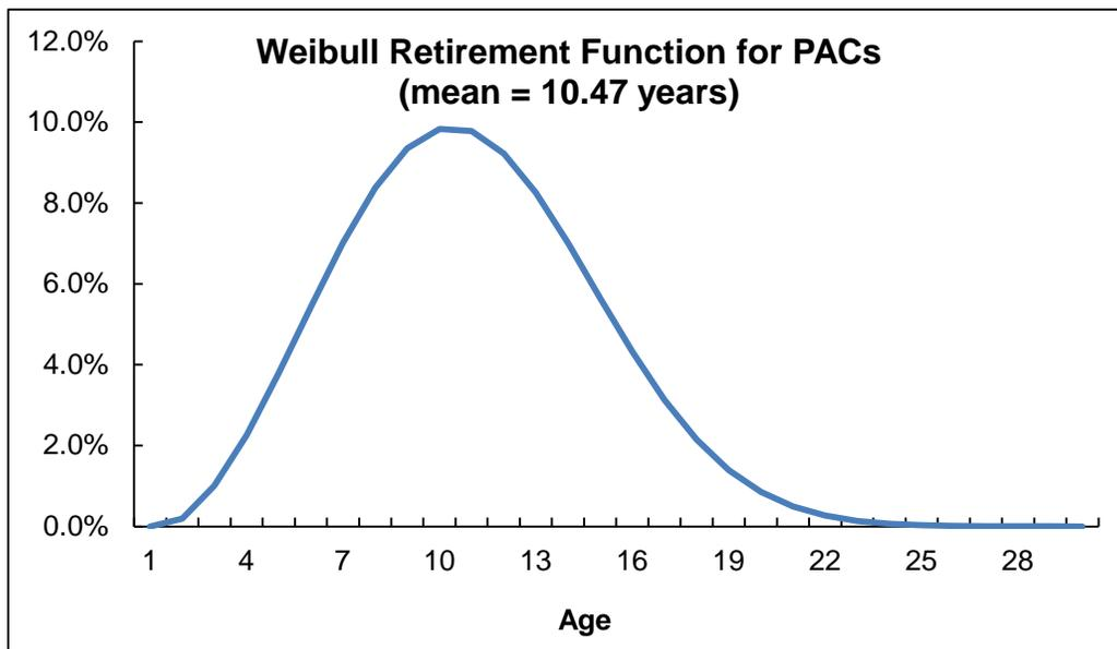
**Figure 8D.3.1 Percent of Portable ACs Retiring each Year**
