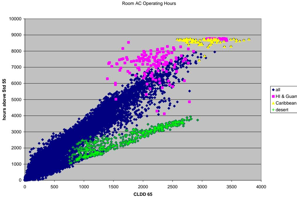
**Figure 7B.3.4 Hours that Exceeded ASHRAE Standard 55 Comfort Zone versus-CLDD Highlighting Various Regions**
