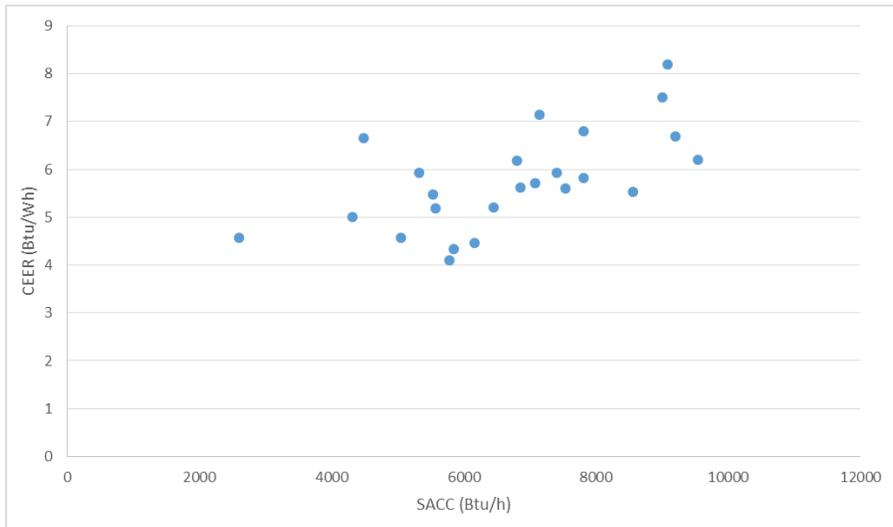
**Figure 5.5.2.3 Test Sample SACC and CEER – Final Rule**
