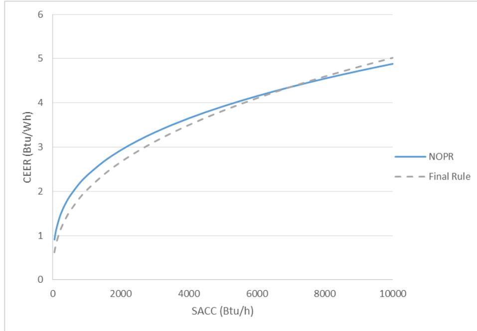
**Figure 5.3.1.3 Baseline Efficiency Levels – NOPR and Final Rule**
