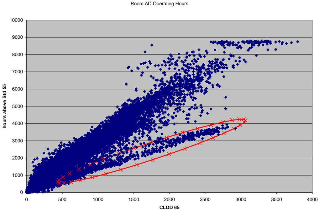
**Figure 7B.3.3 Hours that Exceeded ASHRAE Standard 55 Comfort Zone Compared to CLDD**
