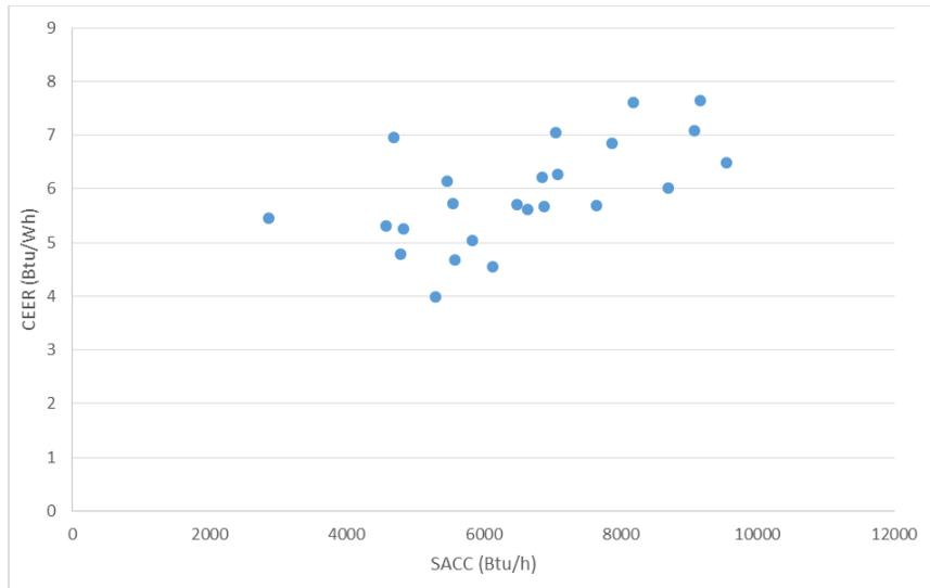
**Figure 5.5.2.2 Test Sample SACC and CEER – June 2016 NOPR**
