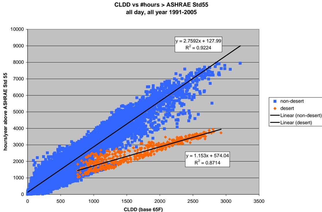
**Figure 7.3.1 Number of Hours that Exceed ANSI/ASHRAE Standard 55 as a Function of Cooling Degree-Days**
