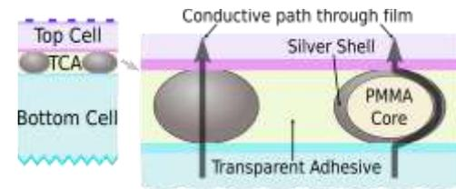
Flexible Microspheres Provide Electrical Connection Between Surfaces Without Lateral Conduction
