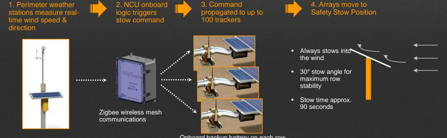
Onboard backup battery on each row ensures reliable stowing
