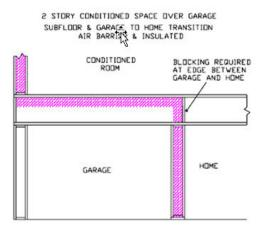
Figure RA3.5-11 Homes with Conditioned Space Over Garage – Insulated Concrete Form (ICF)
