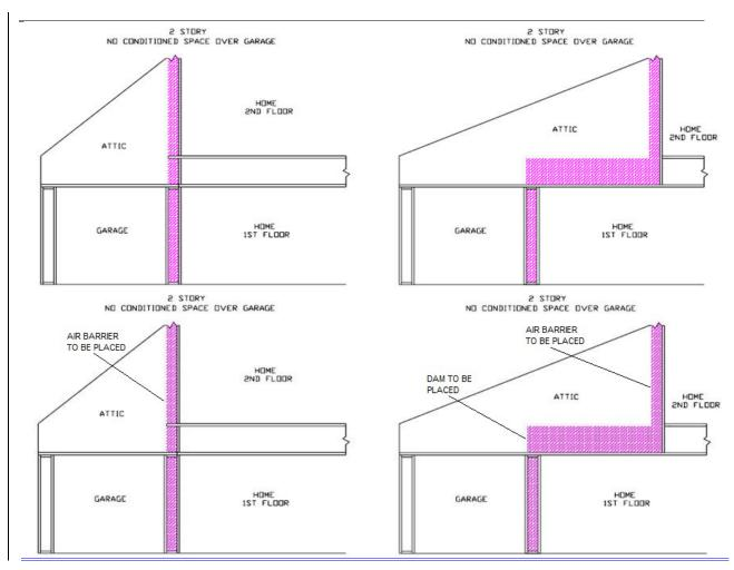
Figure RA3.5-8 Homes with No Conditioned Space Over Garage – Spray Polyurethane Foam Insulation
