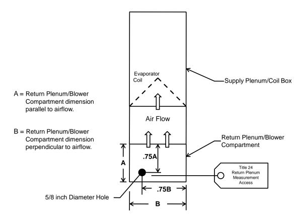
Figure RA3.2-1 Measurement Access Hole
