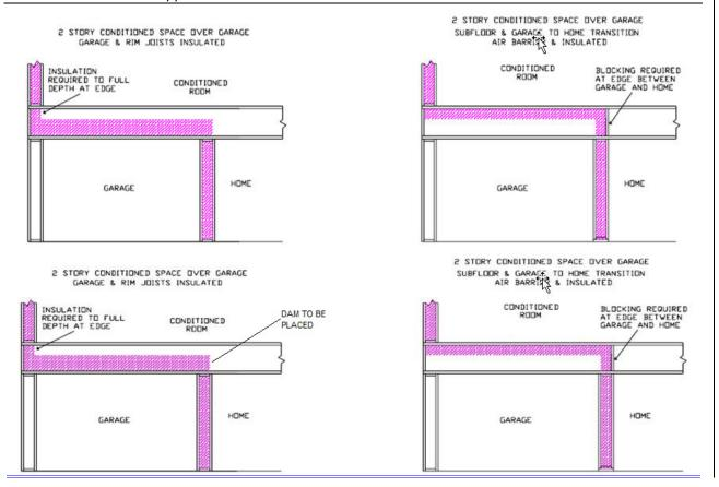
Figure RA3.5-7 Homes with Conditioned Space Over Garage – Spray Polyurethane Foam Insulation
