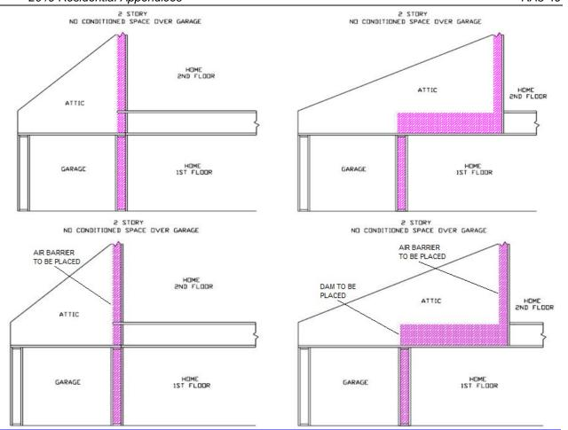
Figure RA3.5-2 Homes with No Conditioned Space Over Garage – Batt and Blanket Insulation
