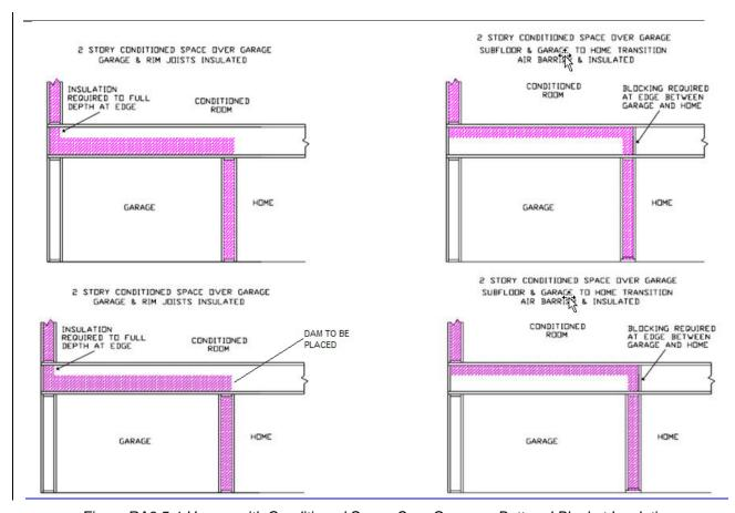
Figure RA3.5-1 Homes with Conditioned Space Over Garage – Batt and Blanket Insulation
