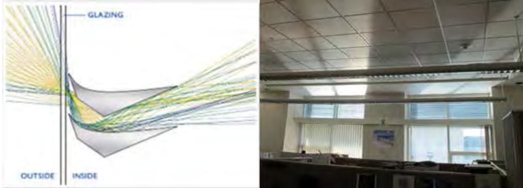
Figure 9: LightLouver profile and field installation
