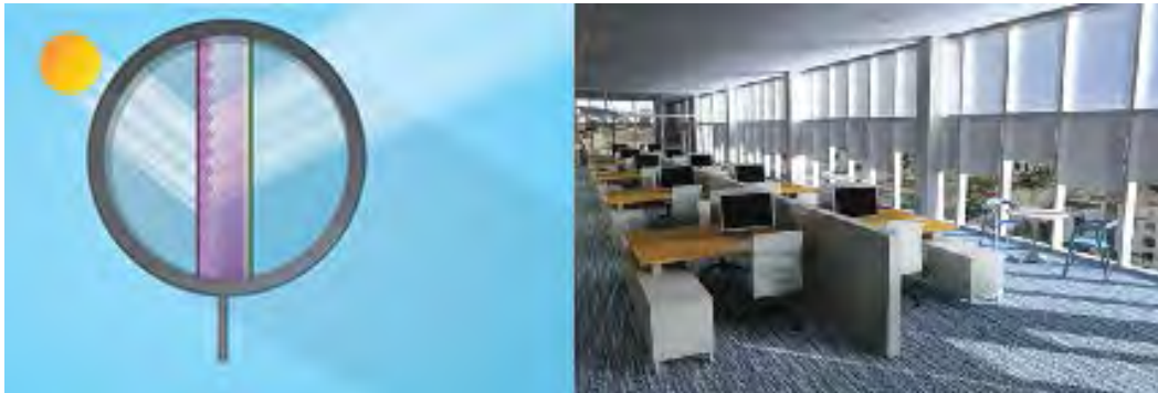
Figure 10: 3M daylight redirecting film profile and field installation
