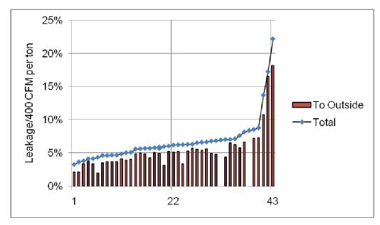
Figure 24: Duct Leakage for Single Family Buildings
