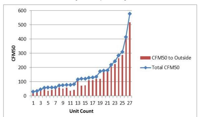
Figure 56: Fireplace Leakage
