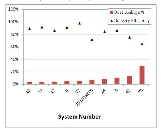
Figure 31: Delivery Efficiency and Duct Leakage
