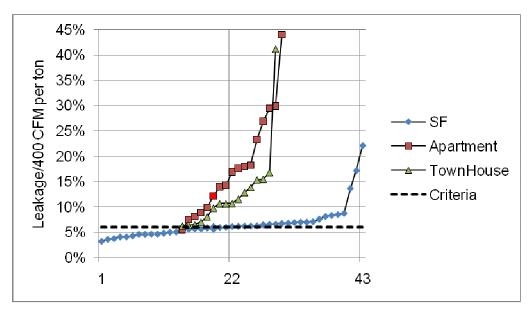
Figure 23: Duct Leakage by Building Type
