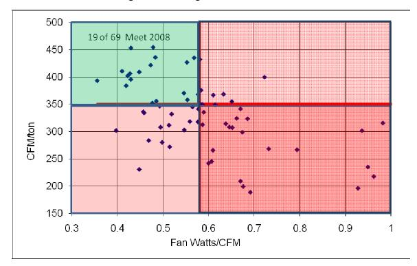
Figure 12: Cooling Airflow and Fan Power
