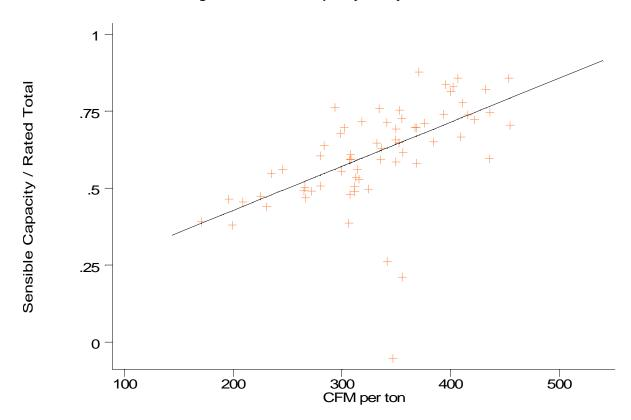
Figure 9: Sensible Capacity vs. System Airflow
