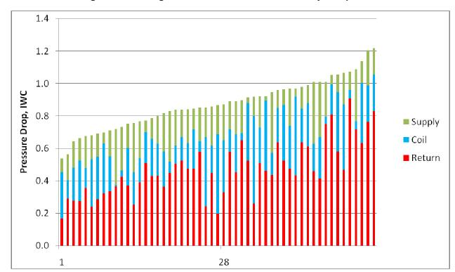
Figure 14: Cooling Airflow External Static Pressure by Component
