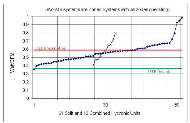
Figure 11: Cooling System Circulating Fan Power
