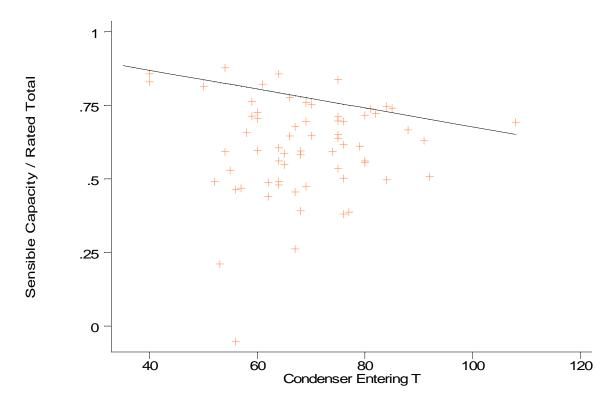
Figure 8: Sensible Capacity vs. Outdoor Temperature
