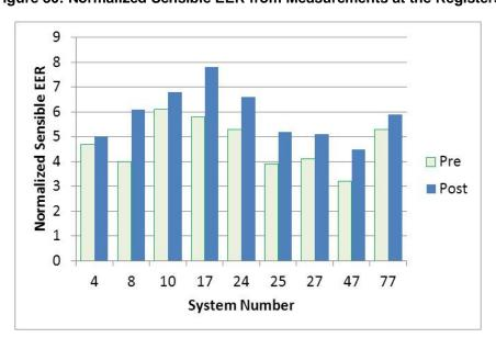
Figure 30: Normalized Sensible EER from Measurements at the Registers
