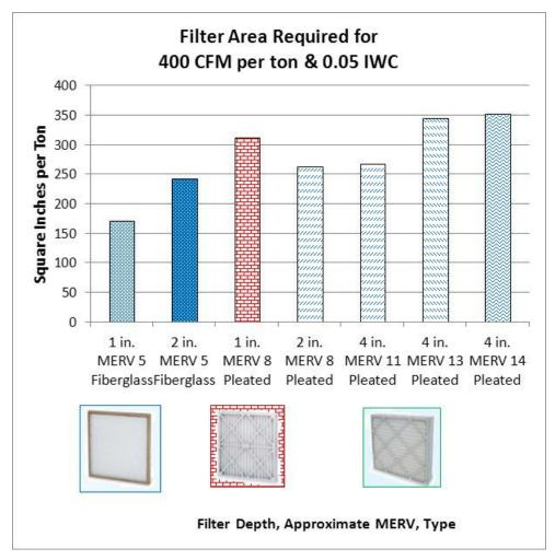
Figure 62: Required Air Filter Area for 400 CEM per Ton at 0.50 IWC
