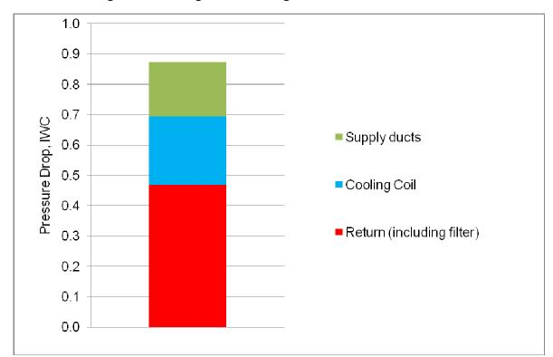
Figure 13: Cooling Airflow Average External Static Pressure
