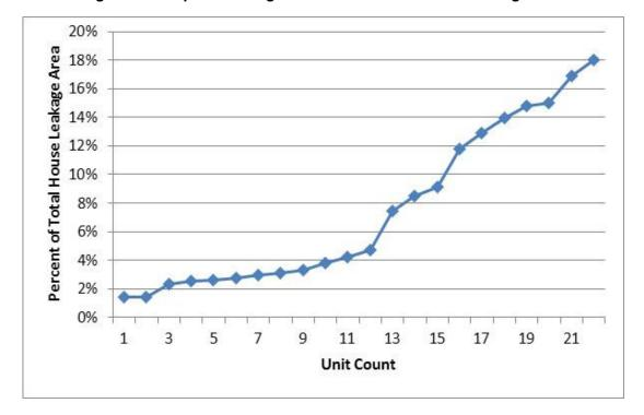
Figure 57: Fireplace Leakage as Percent to Total House Leakage Area
