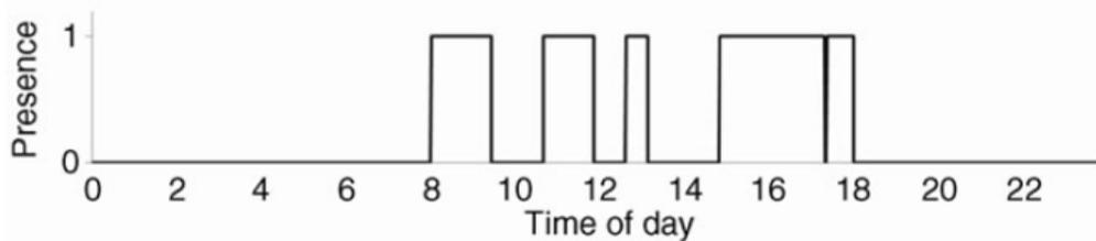
**Figure 35: An example of occupant presence graphed over a 24-hour day.**
