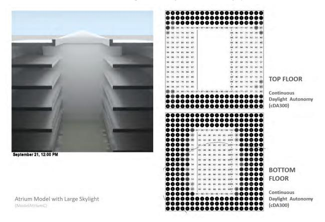
Figure 20: Skylight option (a) 30' x 50' Radiance simulation results
