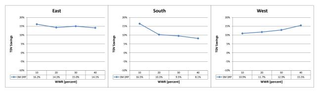
Figure 52: 3M DRF TDV energy savings by WWR
