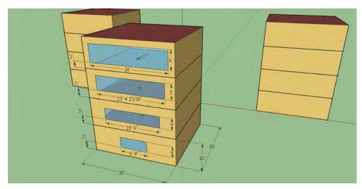
Figure 1: View-window-only prototypes' basic geometry
