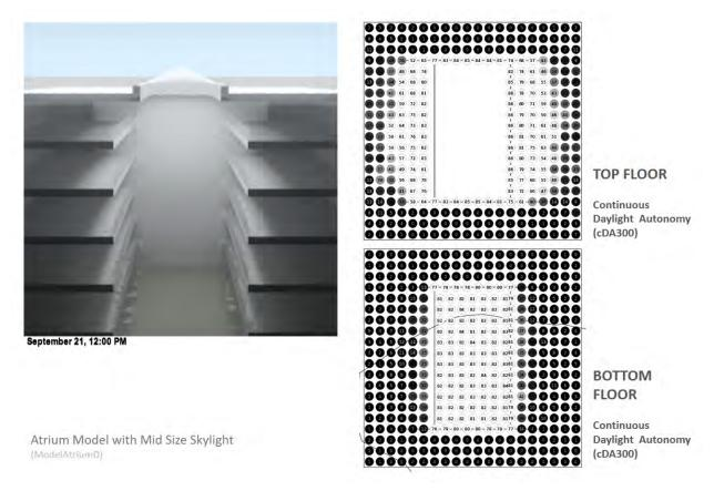
Figure 21: Skylight option (b): 20' x 50' Radiance simulation results
