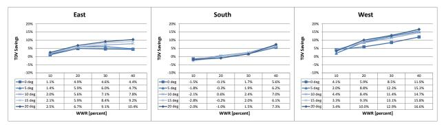
Figure 41: Slat TDV energy savings by WWR and slat angle
