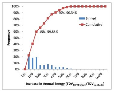
Figure 64: Shades never closed versus 1% VT diffusing shades always closed
