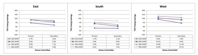
Figure 45: Slat TDV energy savings by zones controlled
