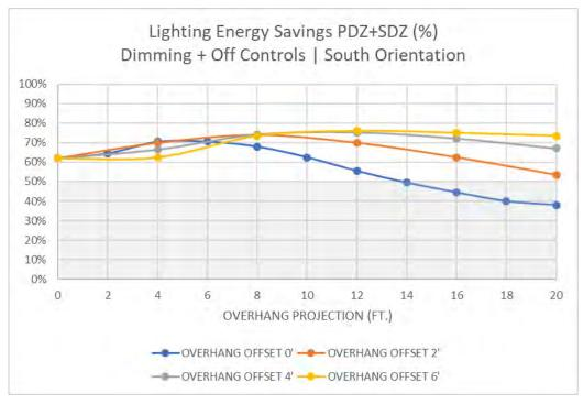
Figure 35: Analysis Set 2 - lighting energy savings plotted against Overhang Projection
