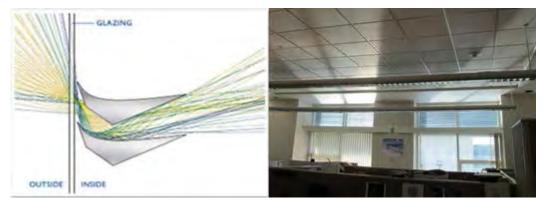
Figure 9: LightLouver profile and field installation
