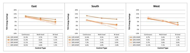
Figure 49: Clerestory TDV energy savings by lighting control type, base case of continuous dimming
