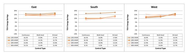
Figure 56: 3M DRF TDV energy savings by lighting control type, same controls in base case
