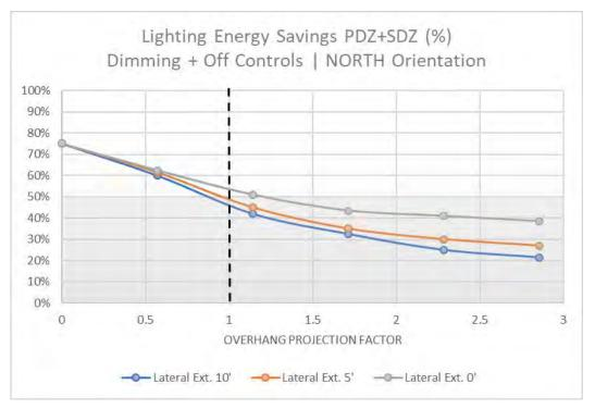
Figure 38: Analysis Set 3 – north window lighting energy savings
