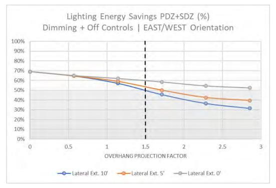
Figure 39: Analysis Set 3 – east/west window lighting energy savings
