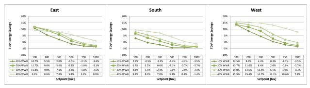
Figure 43: Slat TDV energy savings by lighting control setpoint
