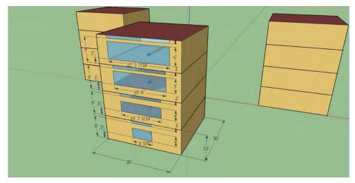
Figure 2: View window with clerestory prototypes' basic geometry
