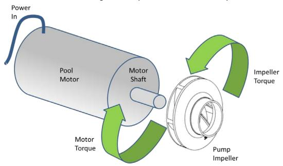
Figure 6-1: Impeller and Motor Shaft Torque
