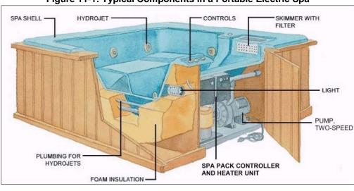
Figure 11-1: Typical Components in a Portable Electric Spa
