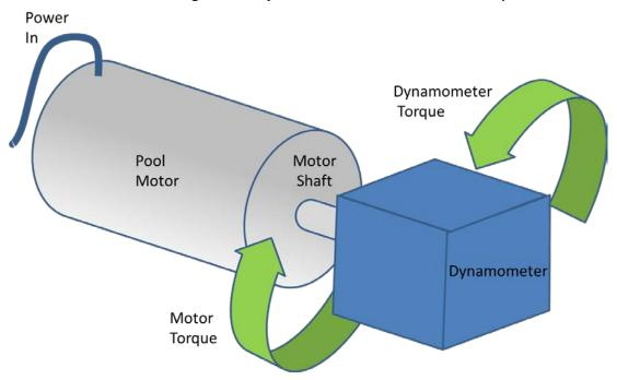
Figure 6-2: Dynamometer and Motor Shaft Torque
