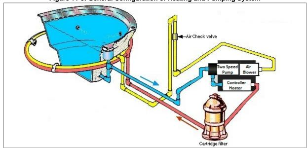
Figure 11-5: General Configuration of Heating and Pumping System
