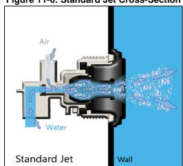
Figure 11-6: Standard Jet Cross-Section
