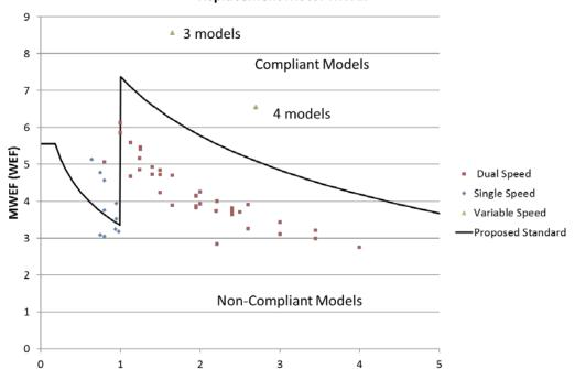
Figure 6-4: MWEF Scores for Replacement Residential Pool Pump Motors
