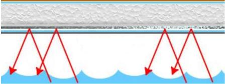
Heat flow being reflected from the radiant barrier.
