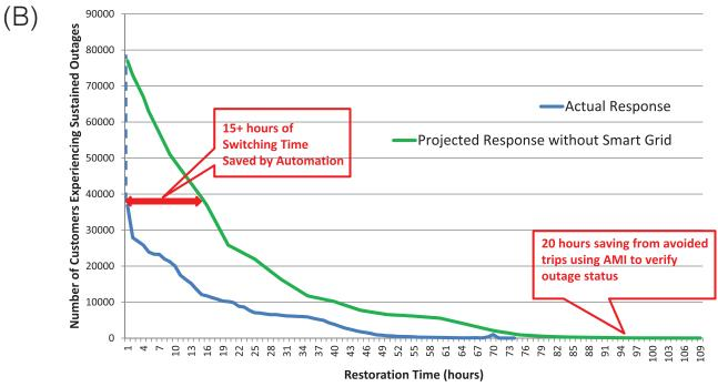
**FIGURE 4.2** (A) Following a major storm that disrupted service on many distribution circuits operated by Chattanooga Electric Power Board, automatic reconfiguration prevented outages for many customers (purple) and significantly reduced the number of circuits requiring manual repairs (green); and (B) such automation has greatly reduced the number of customer-hours (area under the curve) of outage experienced. NOTE: AMI, advanced metering infrastructure. SOURCE: Glass (2016).
