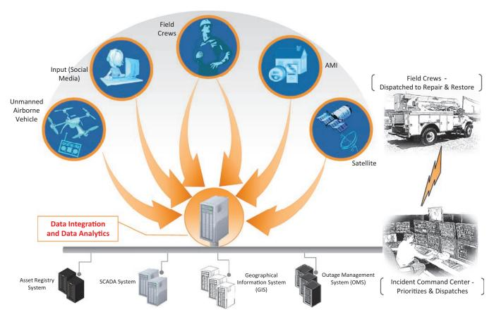
**FIGURE 6.2** Example of data integration to support advanced data analytics for improved restoration efforts. The image above is not comprehensive and other technologies—for example, real-time asset health monitoring equipment and manned airborne vehicles—can be used to collect and relay information on the health of transmission and distribution system components.
