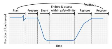
**FIGURE 3.14** Notional time series of a major power outage divided into six stages. The length of each stage and the activities performed by utilities and others involved in the response vary for different disruptions.
