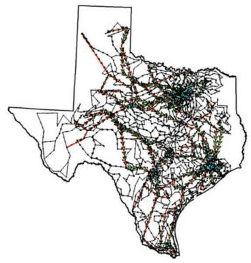
**FIGURE 4.4** 2000-bus synthetic network sited in Texas. The red lines show 345 kV transmission lines, the black lines show 115 kV lines, and the green arrows show the flow of power from the generators to the loads. SOURCE: © 1969 IEEE. Reprinted, with permission, from *Power Systems, IEEE Transactions on Grid Structural Characteristics as Validation Criteria for Synthetic Networks*.
