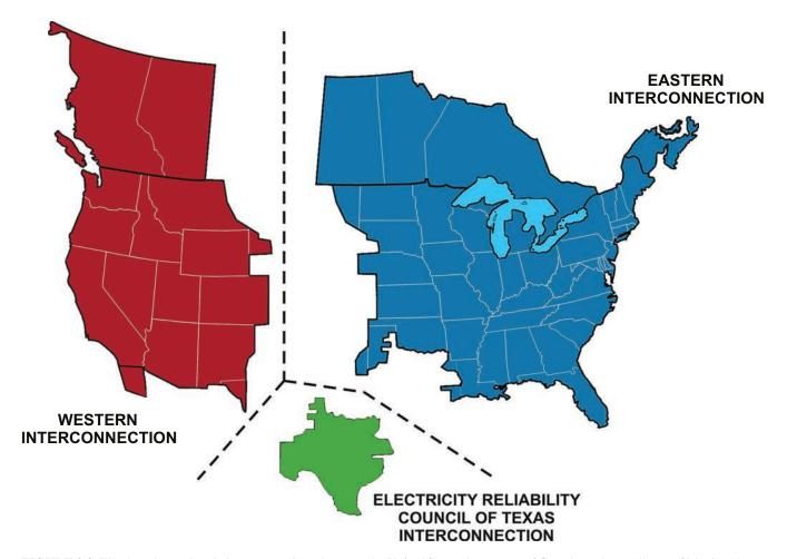
**FIGURE 2.3** The three large electric interconnections that span the United States, large parts of Canada, and a small part of Mexico. A very modest amount of power flows among these three regions over direct current cables so that the 60 Hz power is not synchronized among the regions. Hydro Québec, which is not shown, provides power to many states in the northeastern United States. SOURCE: DOE (2016a).
