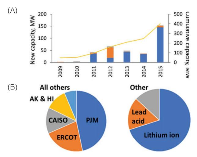
**FIGURE 4.3** (A) Installations of utility-scale battery storage have increased substantially over the past 5 years, (B) although growth is concentrated in a few areas and dominated by lithium-ion chemistries.
