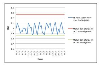
Figure 4 — Data Center Continuous (DCC) system vs. ISO Continuous (COP) system
