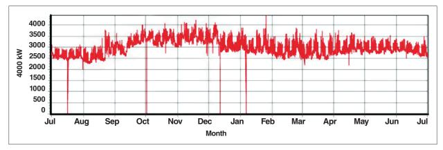
Figure 2 — Typical data center load profile
