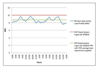
Figure 3 — Data Center Continuous (DCC) system vs. ISO Prime (PRP) system
