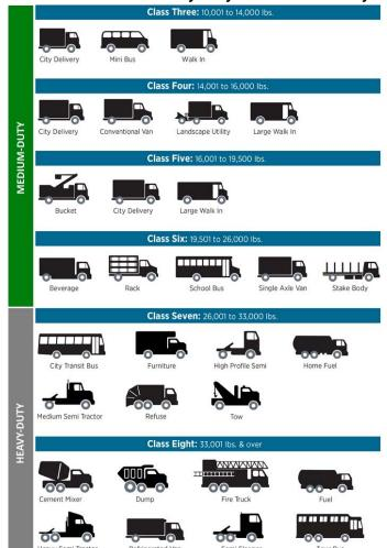
Figure 4-12: Medium- and Heavy-Duty Vehicle Classes by GVWR
