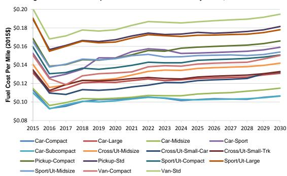
Figure 4-22: Fuel Cost per Mile of Gasoline Vehicles by Class, Mid Case
