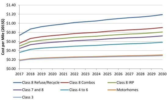
Figure 4-24: Fuel Cost per Mile of Diesel Trucks by Class, Mid Case
