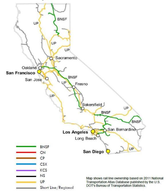
Figure A-4: Rail Routes into and Within California
