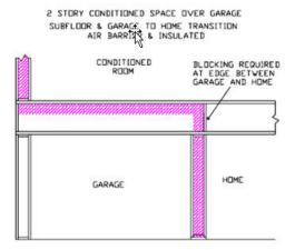
Figure RA3.5-7 Homes with Conditioned Space Over Garage – Spray Polyurethane Foam Insulation
