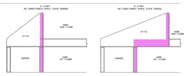
Figure RA3.5-8 Homes with No Conditioned Space Over Garage – Spray Polyurethane Foam Insulation
