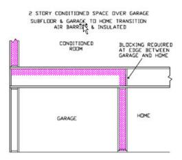
Figure RA3.5-11 Homes with Conditioned Space Over Garage – Insulated Concrete Form (ICF)
