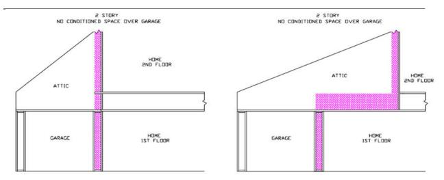
Figure RA3.5-12 Homes with No Conditioned Space Over Garage – Insulated Concrete Form (ICF)
