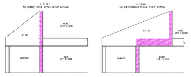
Figure RA3.5-10 Homes with No Conditioned Space Over Garage – Structural Insulated Panel (SIP)
