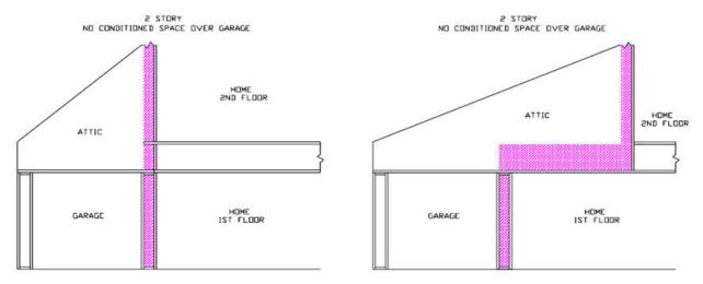
Figure RA3.5-4 Homes with No Conditioned Space over Garage - Loose Fill Insulation
