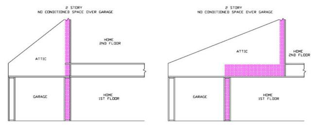
Figure RA3.5-6 Homes with No Conditioned Space Over Garage – Rigid Board Insulation
