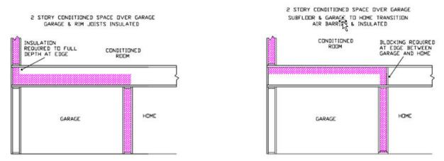
Figure RA3.5-9 Homes with Conditioned Space Over Garage – Structural Insulated Panel (SIP)
