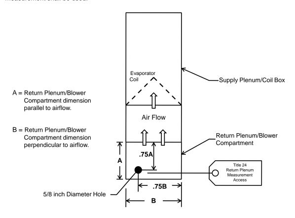
Figure RA3.2-1 Measurement Access Hole
