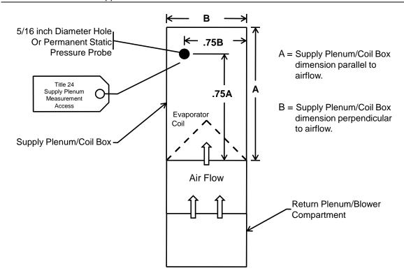
Figure RA3.3-1 Hole for the Placement of a Static Pressure Probe (HSPP) or Permanently Installed Static Pressure Probe (PSPP)
