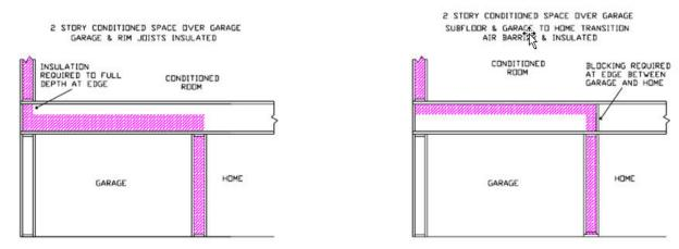
Figure RA3.5-5 Homes with Conditioned Space Over Garage – Rigid Board Insulation
