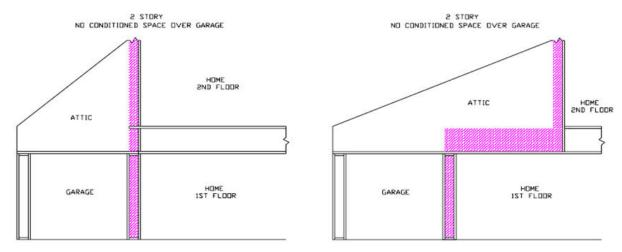
Figure RA3.5-2 Homes with No Conditioned Space Over Garage – Batt and Blanket Insulation
