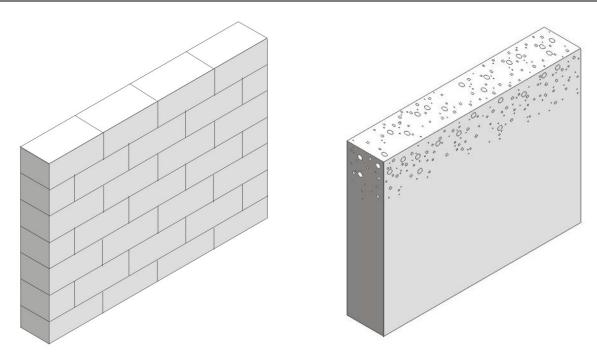
Figure 4.3.6 - Solid Unit Masonry (left) and Solid Concrete (right) Walls
