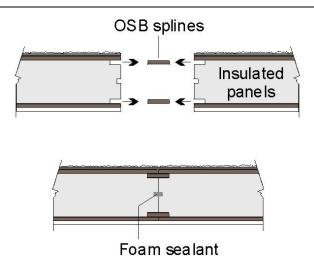
Figure 4.2.4 - SIPS Roof/Ceiling
