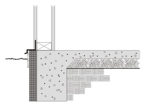
Figure 4.4.8 – Heated Slab-on-Grade Floor
