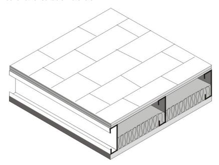
Figure 4.2.6 – Metal Framed Rafter Roof
