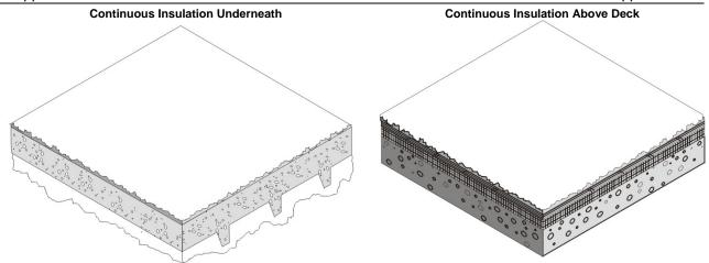
Figure 4.4.6 – Concrete Raised Floors
