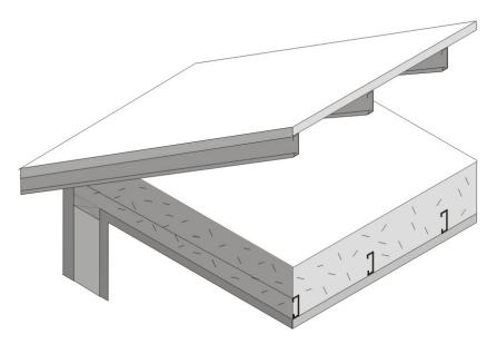
Figure 4.2.5 – Metal Framed Attic Roofs
