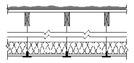
Figure 4.2.9 - Insulated Ceiling with Removable Panels
