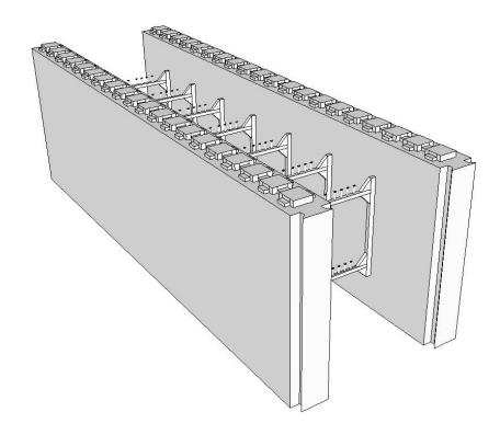
Figure 4.3.13 – Insulating Concrete Forms
