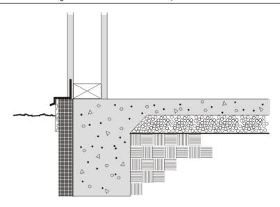
Figure 4.4.7 – Unheated Slab-on-Grade Floor
