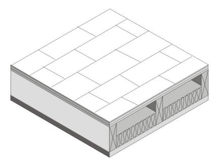
Figure 4.2.3 – Wood Frame Rafter Roof
