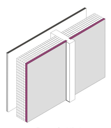
Figure 4.3.8 – Spandrel Panel
