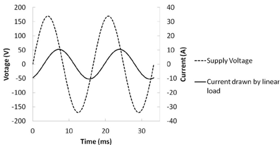
**Figure 1: Linear load exhibiting displacement power factor**
