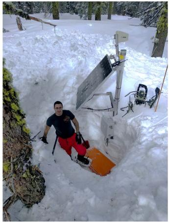
Wireless sensor networks track representative patterns of water content based on physiographic variables.
